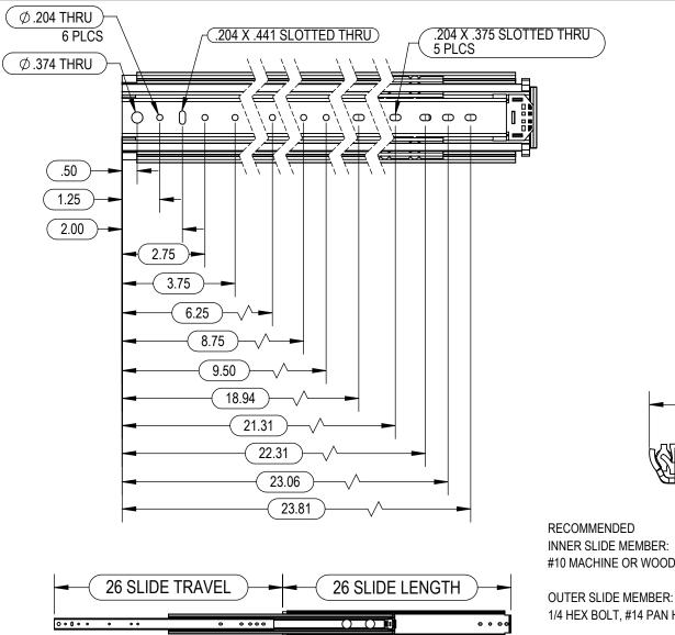
1/4 HEX BOLT, #14 PAN HEAD WOOD SCREW FOR ALL THRU HOLES AND SLOTTED THRU HOLES
